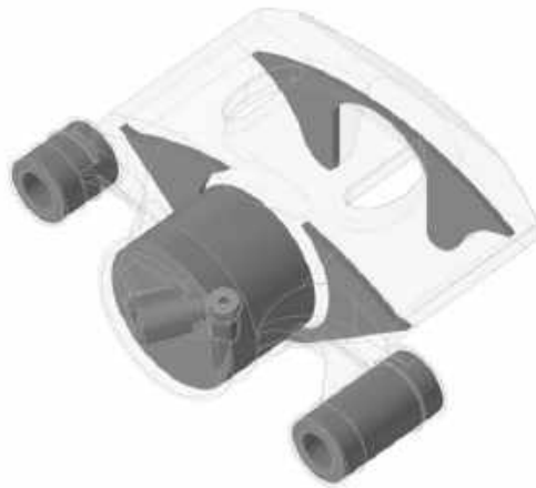
Fig 12. Undesigned area of brake caliper.
