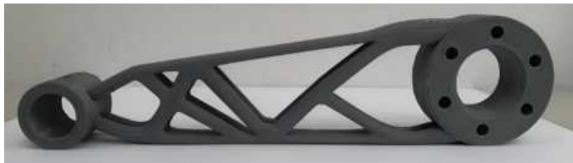
Fig 3. 3D printed model of optimal design ( Tran Thanh Hai Tuan, 2020)
