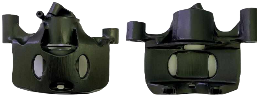
Fig 20. 3D printed model of the optimal design
